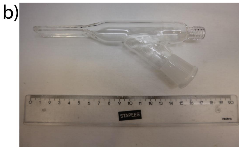
Figure S1. SI-PET-RAFT polymerization setup (a), photo-polymerization reactor (b)
