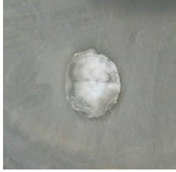
Fig.S2. The antibacterial activity of pure PVA sample against S. aureus . The experiment shows no antibacterial activity for this specimen against the mentioned bacteria.
