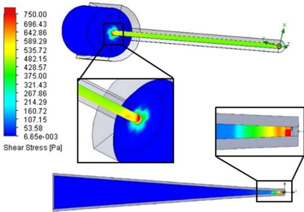
501 **Supplemental Figure II:** Computational modeling of flow in 200µm conical and cylindrical needles at 3.5 bar. Heat maps of the simulated fluid flow induced shear stresses for both needle types.
