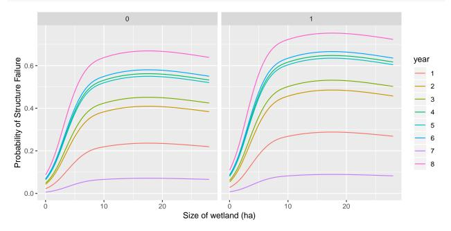
Get predictions averaged across years. We see that failure rates were slightly higher in double-cylinder than single-cylinder structures.
