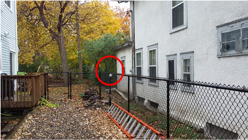
SI Fig. 2: Sample of the low-cost sensor set up (within the red circle) in St. Anthony Park. In each neighborhood, monitors were ziptied to fences or other stationary spots outside the house that were isolated and away from emission sources. Monitors were elevated to approximately the inhalation height in each neighborhood.
