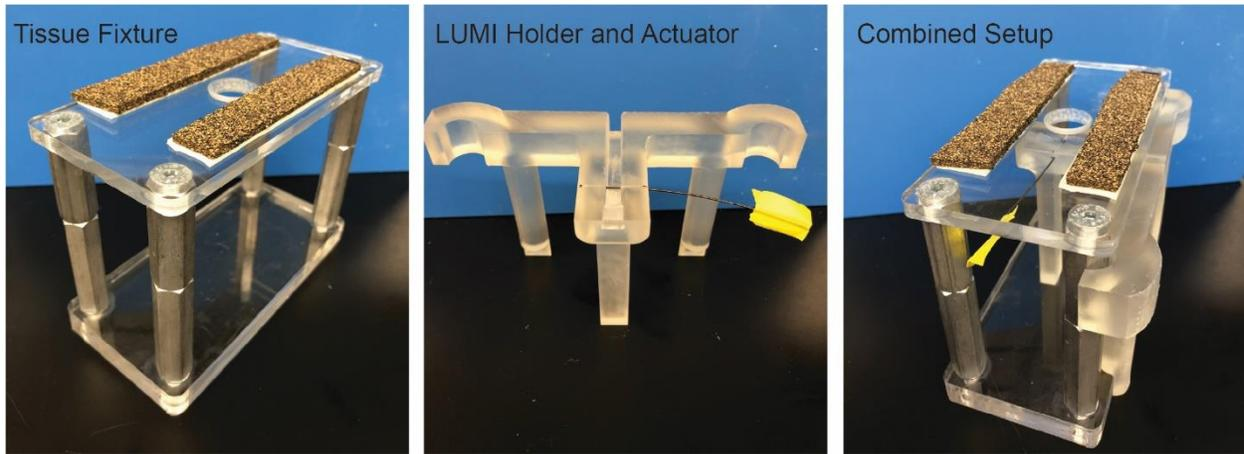
**Supplementary Fig. S15** Fixture used to release LUMI *ex vivo* for OCT imaging. The tissue was fixed to the top section of the fixture using push pins. Two LUMI arms were fixed using the LUMI holder and another arm was placed underneath the wire (marked with yellow tape). The LUMI holder was then placed under the tissue fixture. The arm was then released and allowed to unfold after removing the wire.
