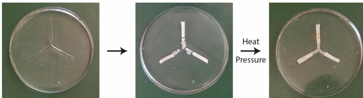
**Supplementary Fig. S14** LUMI fabrication process. Custom fabricated PDMS mold for creation of LUMI backbone. We used Mediprene for the elastomer core and a PEO/Soluplus<sup>®</sup> mixture for the arms. Metal cores were embedded in the elastomer during heating.
