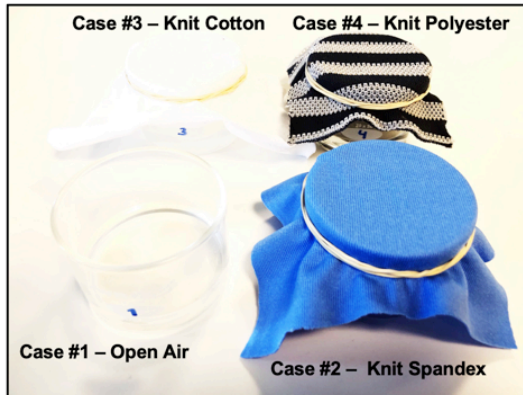
Supplementary Figure 14: Water vapor evaporation rate setup. a) Three different fabrics and an open air (control) under test, b) Accumulated weight change of liquid content in grams per day on every sample.
