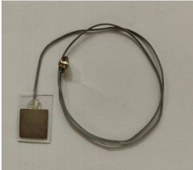
Figure S2 Shows the AgNW/PDMS dry electrode with wire and metal snap.
