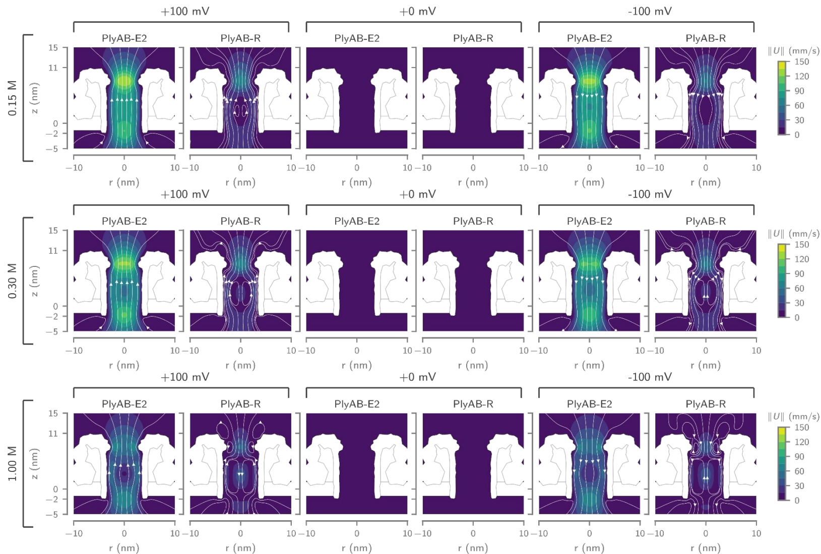
Figure S15. Water velocity distribution in PlyAB-E2 and PlyAB-R at 0.15 M, 0.3 M and 1.0 M NaCl bulk reservoir concentrations and at +100 mV, 0 mV and -100 mV applied bias potentials.
