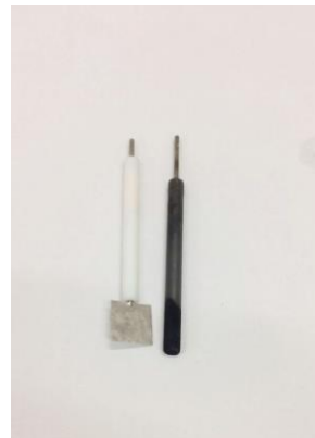
C) Carbon rod anode and platinum plate cathode
