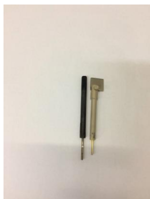
D) Carbon rod anode and nickel plate cathode
