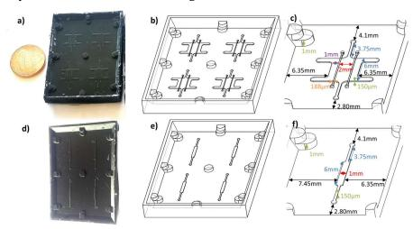
Figure 2. SolidWorks designs and corresponding pictures of the different molds employed to fabricate the two devices: (a–c) For the cell culture experiments and (d–f) the oxygen diffusion characterization.
