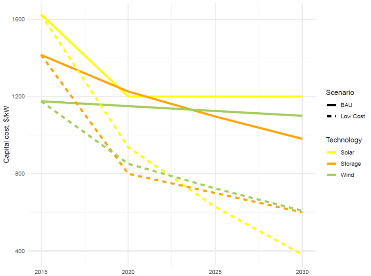
Supplementary Fig. 2 Capital costs of wind, solar, and storage technologies under BAU and Low Cost scenarios (R), 2015 to 2030. Capital costs of wind, solar, and storage technologies in the Carbon constraint scenario (C50) and Carbon constraint scenario (C80) are the same as in the Low Cost scenario (R).
