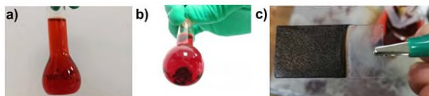
Figure S17. Photos of \text{Ru}^{\text{II}}\text{XY} solutions before (a) and after (b) iterative synthesis, and photo of bare ITO electrode without pre-assembled molecule after electrolysis of \text{Ru}^{\text{II}}\text{XY} at 1.0 V for 1h (c). The precipitation can be found after iterative synthesis, indicating the oligomers become insoluble, and also implying that the single organometallic polymer with 10 units will be hard to be soluble. After
