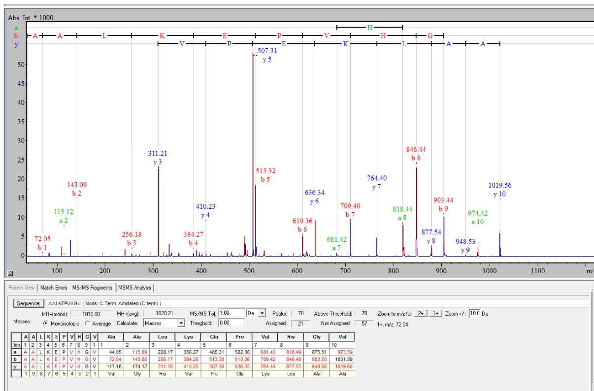
Supplementary Figure 99. MALDI-TOF-TOF sequencing of AALKEPVHGV-NH 2 peptide. Matrix \alpha -cyano-4-hydroxycinnamic acid, positive detection mode. The MS-MS analysis confirms that the SetAla residue is converted into the Ala amino acid in the peptide.
