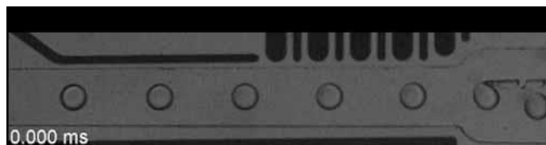
Movie S4. High-speed imaging of the sorting process of the SADA sorter (The volume of sorted droplets: 1 nL). Cell-encapsulating droplets (1 nL in volume) were sorted from a mixture of cell-encapsulating and numerous empty droplets at the
