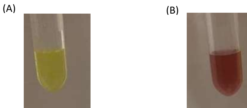
Figure S2: Photograph of gold dispersion (A) before and (B) after GNPs formation by the Turkevich method. For NPs preparation, HAuCl 4 solution (100mL) was boiled in a conical flask under continuous stirring followed by addition of 1% w/v sodium citrate aqueous solution (10mL). Heating under reflux with stirring continued till formation of a red color.
