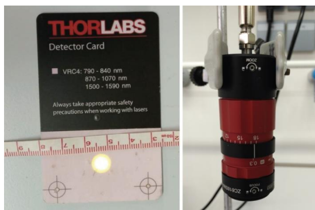
Figure S13. Image of spot diameter using a NIR detector card (left) and the collimation/zoom system (right).
