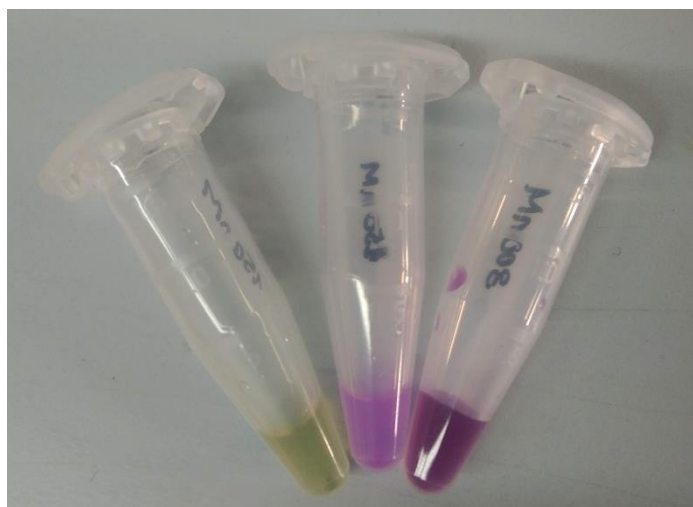
Figure S8. UC-PMA NPs conjugated with one PS type: from left to right, Chlorin e6 (UC-PMA-Ce6), Rose Bengal (UC-PMA-RB) or both PS. (UC-PMA-RB,Ce6)
