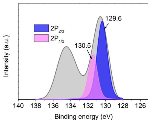
**Supplementary Figure 10.** High-resolution XPS P  $2p$  spectra of BPNS that was sprayed on cleaned silicon plates and placed in a normal atmosphere for 24 hours.
