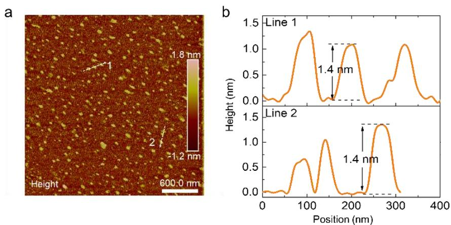
**Supplementary Figure 9.** AFM characterization. (a) AFM image of BP@Cu<sub>0.8</sub> after 24-hour incubation at room temperature. (b) AFM height profile of BP@Cu<sub>0.8</sub> along the two lines in image a.
