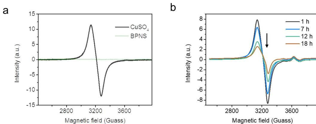
**Supplementary Figure 12.** EPR characterization. (a) EPR spectra of  $\text{CuSO}_4$  and BPNS. (b) EPR spectra of  $\text{BP@Cu}_{0.4}$  obtained at various time points to monitor the redox reaction between BPNS and  $\text{Cu}^{2+}$  at the atmosphere. The decrease in the intensity of  $\text{Cu}^{2+}$  indicates the reduction of  $\text{Cu}^{2+}$  to  $\text{Cu}^{+}$ .
