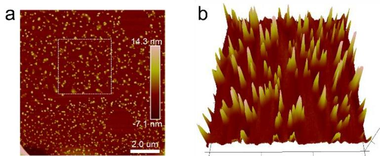
**Supplementary Figure 6.** AFM characterization. (a) AFM image of BP@Cu@PEG-RGD in a large area. The white frame denotes the selected area in Fig. 2g. (b) Three-dimensional morphology of BP@Cu@PEG-RGD. Similar AFM images were observed for more than two times experiments.
