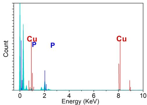
**Supplementary Figure 4.** Energy disperse X-ray spectroscopy analysis of the BPNS. Intense signals from Cu were observed in the spectrum.
