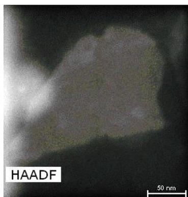
**Supplementary Figure 3.** STEM image of the BP@Cu corresponding to the elemental mapping in Figure 2d-e. Similar STEM images were observed for more than three independent experiments.
