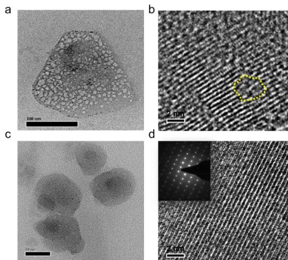
**Supplementary Figure 5.** TEM characterization. (a) TEM images of BP@Cu<sub>0.4</sub>. (b) HR-TEM of BP@Cu<sub>0.4</sub>. The yellow circle indicates the surface oxidation of BPNS. (c) TEM images of BP@Cu<sub>0.4</sub>@PEG-RGD. (d) HR-TEM of BP@Cu<sub>0.4</sub>@PEG-RGD. The inset in d shows the SAED pattern. Similar TEM and HR-TEM images were obtained for three times experiments.
