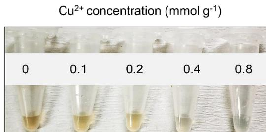
**Supplementary Figure 7.** The optical images of BPNS incubating with different concentrations of  $\text{Cu}^{2+}$  for 48 hours.
