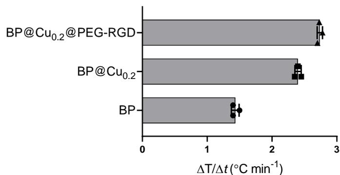
**Supplementary Figure 13.** The corresponding temperature increment per minute for BP, BP@Cu, and BP@Cu@PEG-RGD, respectively. The data represents the mean  $\pm$  s.d.,  $n = 3$  independent experiments.
