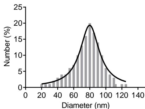
**Supplementary Figure 2.** AFM statistics of the lateral size of BPNS. The data are calculated based on three independent measurements.
