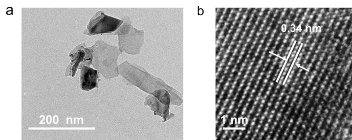
**Supplementary Figure 1.** TEM characterization. (A) TEM images of BPNS. (B) HR-TEM of BPNS and its lattice fringes. Similar TEM and HR-TEM images were obtained for three times experiments.
