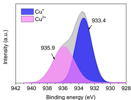
**Supplementary Figure 11.** High-resolution XPS P  $2p_{2/3}$  spectra of Cu. The ratio of  $\text{Cu}^{+}$  and  $\text{Cu}^{2+}$  were simulated. The BPNS was sprayed on cleaned silicon plates and placed in a normal atmosphere for 24 hours.
