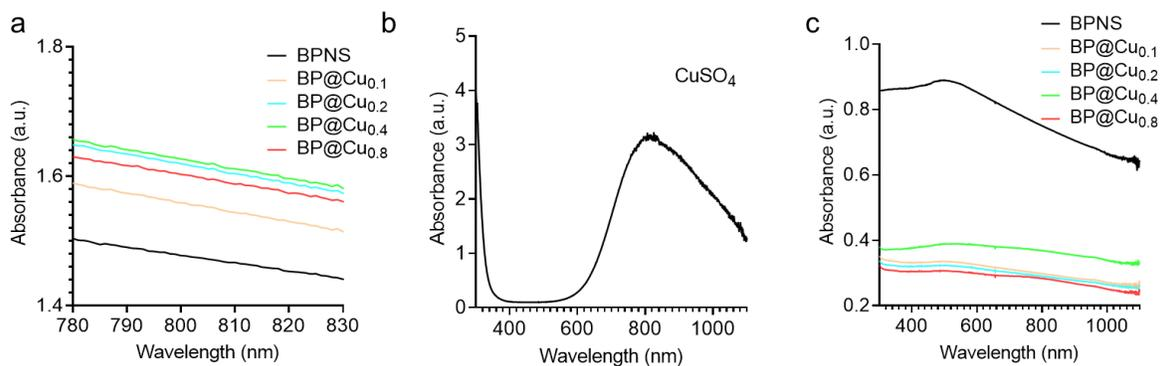
**Supplementary Figure 8.** UV-Vis-NIR characterization. (a) The absorbance spectra of BPNS and BP@Cu<sub>x</sub> in ddH<sub>2</sub>O at the wavelength of 780-830 nm. (b) UV-Vis-NIR absorbance spectrum of 0.25 M CuSO<sub>4</sub> in double-distilled water (ddH<sub>2</sub>O). (c) The absorbance spectra of BPNS and BP@Cu<sub>x</sub> in ddH<sub>2</sub>O after 24 hours incubation at room temperature.
