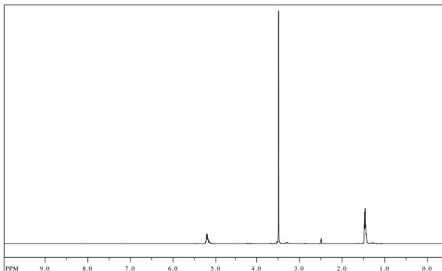
**Figure S9.**  $^1\text{H-NMR}$  (DMSO- $d_6$ , 400 MHz) spectra of  $\text{NH}_2\text{-PEG}_{5\text{k}}\text{-PLA}_{010\text{k}}$ .  $\delta$  (ppm): 1.44 ppm ( $-\text{C}(\text{CH}_3)\text{H}-$ ), 2.50 ppm (solvent peak), 3.30 ppm ( $\text{H}_3\text{COCH}_2\text{CH}_2-$ ), 3.49 ppm ( $-\text{OCH}_2\text{CH}_2-$ ), 4.21 ppm ( $-\text{OCH}_2\text{CH}_2-\text{O}(\text{CO})-$ ), 5.17 ppm ( $-\text{C}(\text{CH}_3)\text{H}-$ ).
