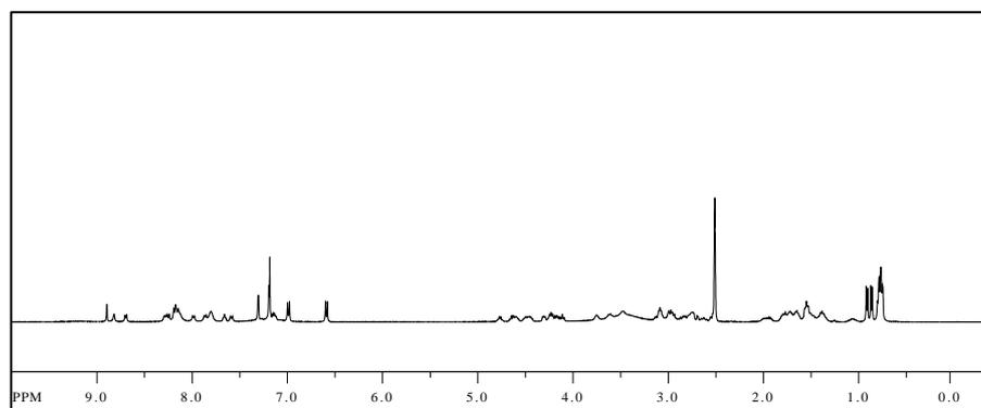
**Figure S13.**  $^1\text{H-NMR}$  (DMSO- $d_6$ , 400 MHz) spectra of Lys-Ang-I.  $\delta$  (ppm): 0.73 ( $-\text{CH}(\text{CH}_3)\text{CH}_3$ ), 0.84 ( $\text{CH}_3-\text{CH}(\text{CH}_3)\text{CHN}$ ), 2.50 (solvent peak), 6.59 ppm ( $=\text{CHC}(\text{H})=\text{CH}$ ), 7.20 ppm ( $=\text{CHC}(\text{H})=\text{CH}$ ), 8.20 ppm  $\text{CO}(\text{NH})\text{CH}(\text{CH}_2)\text{CO}$ .
