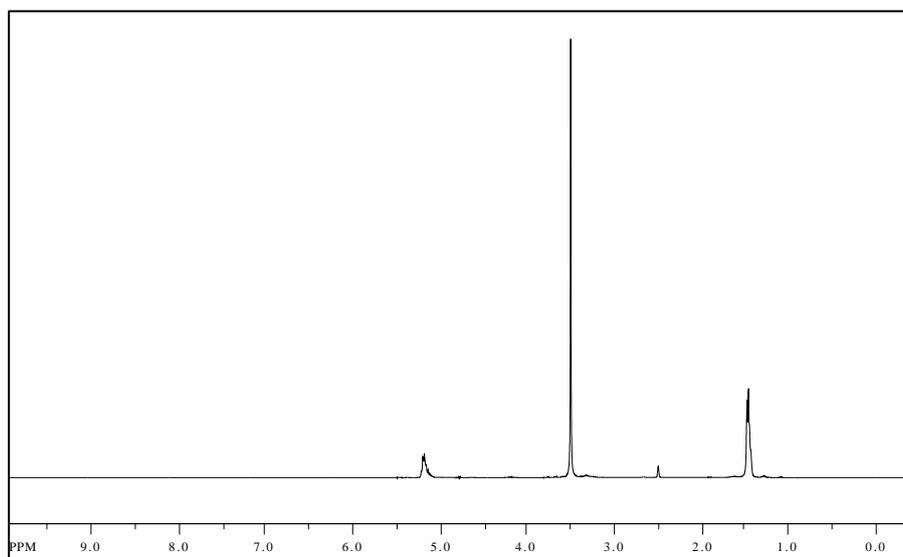
**Figure S12.**  $^1\text{H-NMR}$  (DMSO, 400 MHz) spectra of  $\text{COOH-PEG}_{5\text{k}}\text{-PLA}_{10\text{k}}$ .  $\delta$  (ppm): 1.46 ppm ( $-\text{C}(\text{CH}_3)\text{H}-$ ), 2.50 ppm (solvent peak), 3.30 ppm ( $\text{H}_3\text{COCH}_2\text{CH}_2-$ ), 3.49 ppm ( $-\text{OCH}_2\text{CH}_2-$ ), 4.19 ppm ( $-\text{OCH}_2\text{CH}_2-\text{O}(\text{CO})-$ ), 5.19 ppm ( $-\text{C}(\text{CH}_3)\text{H}-$ ).
