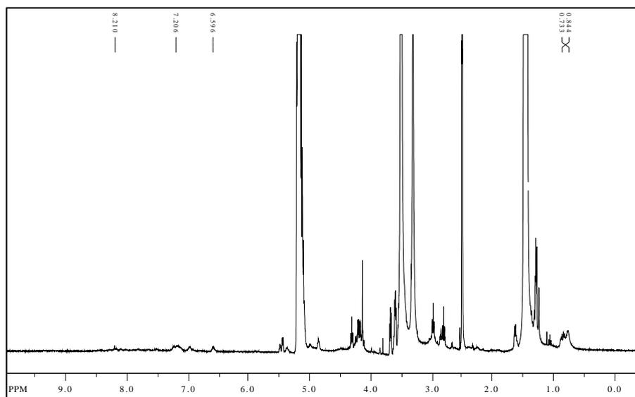
**Figure S14.**  $^1\text{H-NMR}$  (DMSO- $d_6$ , 400 MHz) spectra of Ang-I- PEG $_{5k}$ -PLA $_{10k}$ . Characteristic Lys-Ang-I shifts (marked) confirm the successful coupling of Lys-Ang-I to COOH-PEG $_{5k}$ -PLA $_{10k}$ .  $\delta$  (ppm): 0.73 (-CH(CH $_3$ )CH $_3$ ), 0.84 (CH $_3$ -CH(CH $_3$ )CHN), 2.50 (solvent peak), 6.59 ppm (=CHC(H)=CH), 7.20 ppm (=CHC(H)=CH), 8.20 ppm CO(NH)CH(CH $_2$ )CO.
