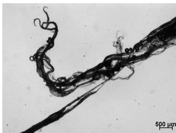
Figure S1. LM photograph of PLGA agglomerates appearing in an EA microsphere suspension. To prepare microspheres, a dispersed phase (250 mg PLGA/70 mg progesterone/3 ml EA) was emulsified in an EA-free aqueous phase. When the emulsion was subject to solvent removal, not only embryonic microspheres but also fiber-like PLGA agglomerates were generated. The bar size is 500 \mu\text{m} .
