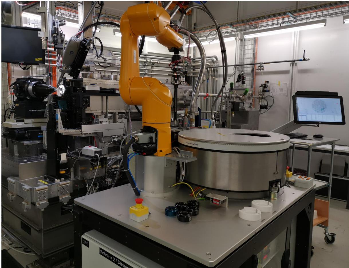
**Figure S3** Picture of TELL installed at X10SA-PXII, Swiss Light Source. Elements are described in Figure 1 of the main manuscript.
