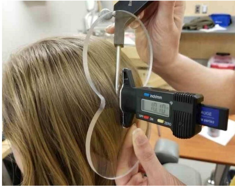
Figure S4. Illustration of the process of measurement of compressed hair thickness.
