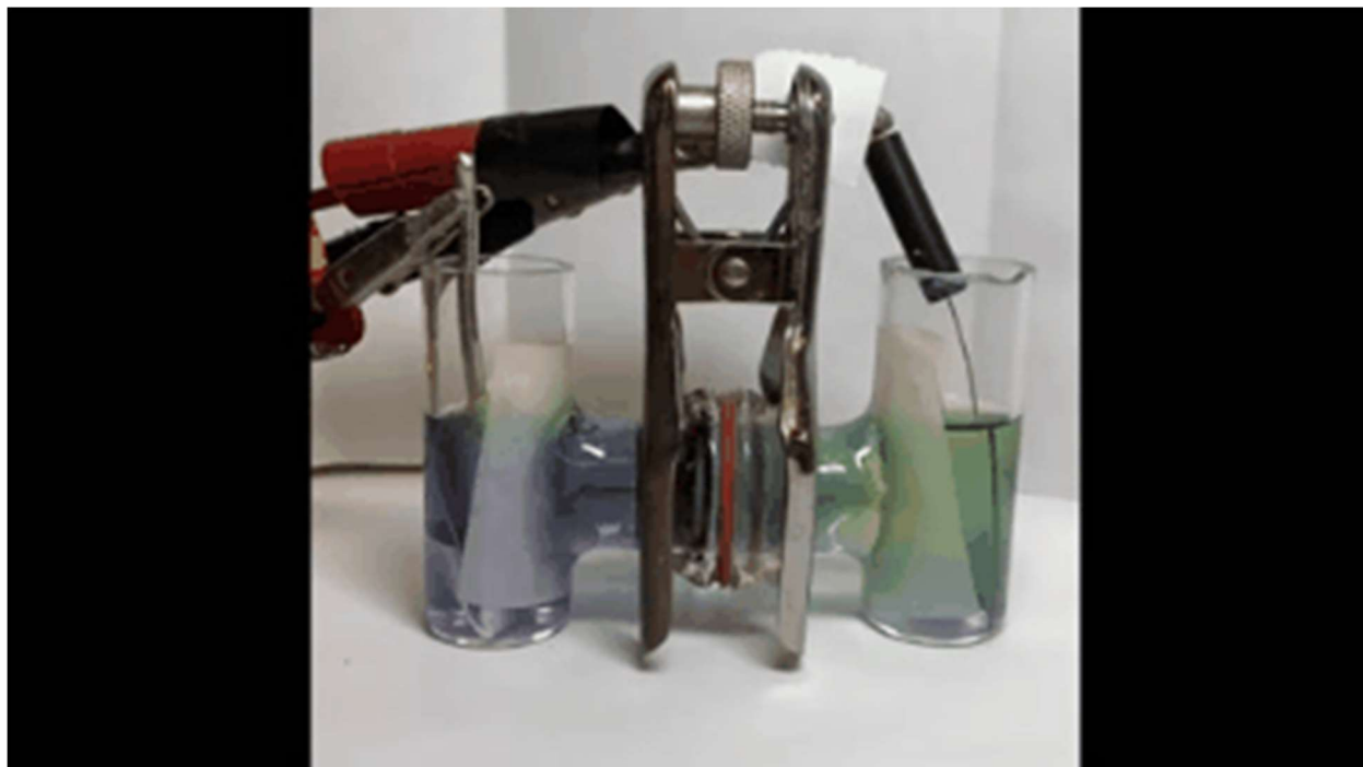
Video V2. [See separate video file] Time-lapse video of the decarbonation cell containing pH indicator dye, shown in Figure 3F-H. Porous paper separators have been placed in front of each electrode as shown schematically in Figure S1B, and CaCO 3 powder in a cup surrounding the OER electrode on the left.
