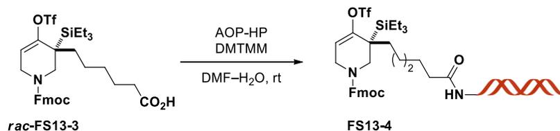
**FS13-4** was synthesized from *rac*-**FS13-3** as described for the preparation of **11** and isolated by preparative HPLC (74% yield by photospectrometry).
