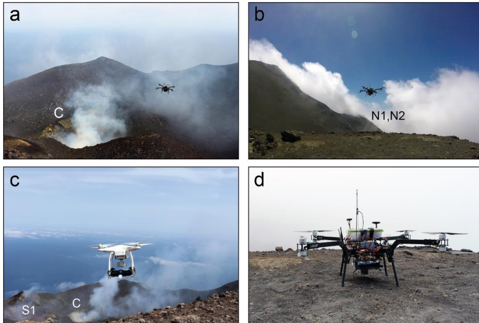
Supplementary Figure 3: Unoccupied Aerial Systems (UAS) used in this study. (a, b, d) Multi-GAS sensor in upward-mounting position on a Vulcan Black Widow X8 (Vulcan UAV, UK) platform with custom avionics. (c) Aeris (Airgraph, Australia) mounted on a DJI Phantom 3 Pro quadcopter. Takeoff and landing sites included (a, c) Fortini – southwestern rim of crater terrace, and (b, d) La Rochetta – northern rim of crater terrace.
