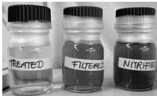
Figure S 8 After the treatment with GAC the urine was almost colorless and odorless
