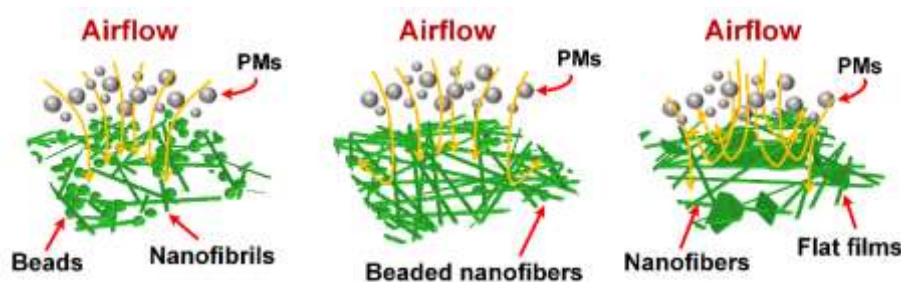
Figure S7. Schematic showing the PM filtration processes using different microparticle/nanofibril, beaded nanofiber, and nanofiber/film membranes.
