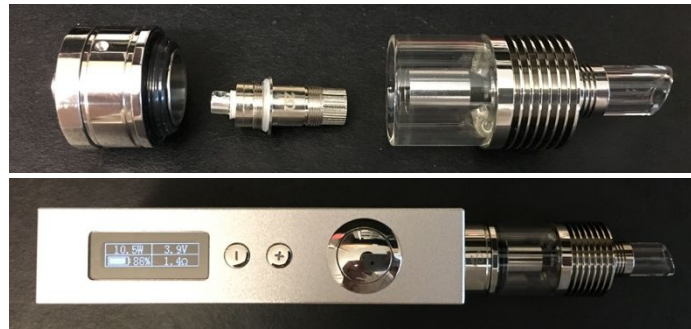
Figure S1. E-cigarette device used in the study: the cartomizer (top) and battery box (bottom)
