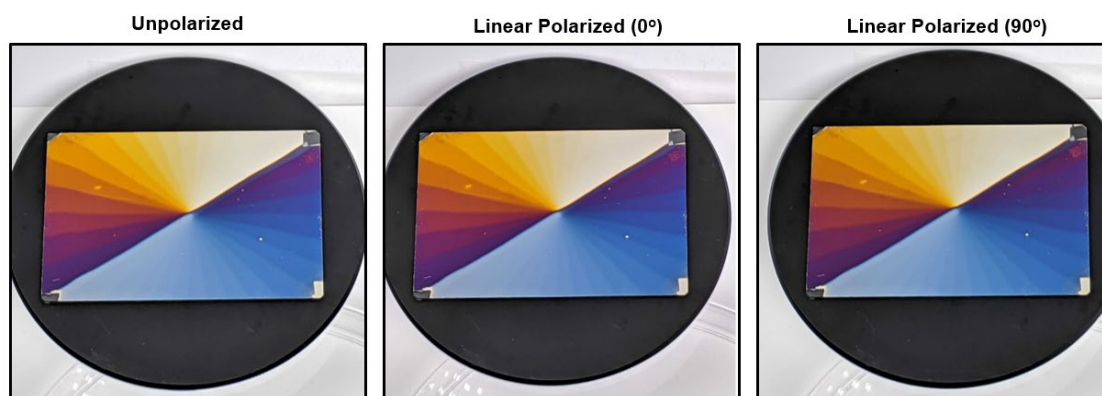
Fig. S3 | Polarization Photography of Plasmonic Surface. Images of the plasmonic surface under unpolarized and linearly polarized states. Linear polarized images are obtained by inserting and rotating a linear polarizer (LPVISE100-A, Thorlabs) in front of a camera (Pixel 3XL, Google).
