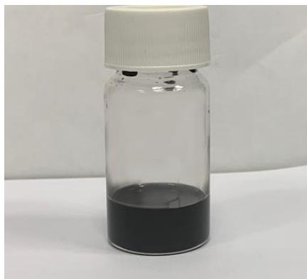
Figure S1. Optical photograph of an 8 week old suspension of diluted CP in isopropanol as used in our experiments to demonstrate the stability of the suspension: no sedimentation could be observed. According to the specifications of the manufacturer, 6 the concentrated CP has an indefinite shelf-life.
