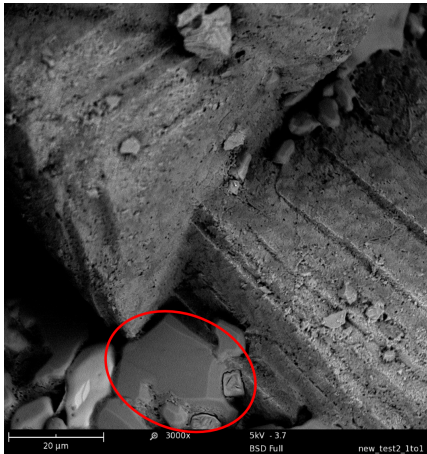
(d) Inter-grown and dodecahedral crystals with pentagonal faces. Magnification: 3000×.
