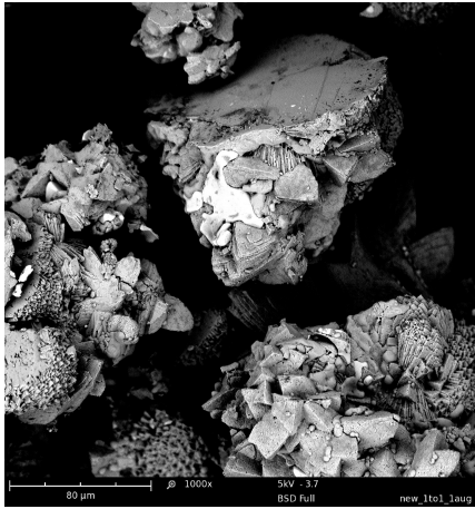
(a) Overview of calcite crystals embedded in an organic matrix. Magnification: 1000×.
