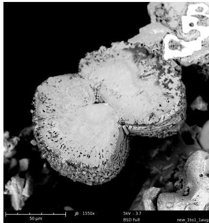
(h) Wheat-sheaf of crystals with starting signs of a hollow core. Magnification: 1550×.
