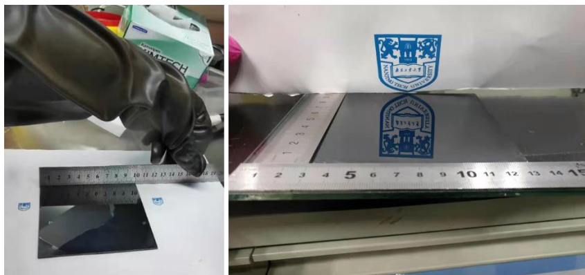
Figure S5 Photograph of the 10mm ×10mm large-scale perovskite films treated by MAP.
