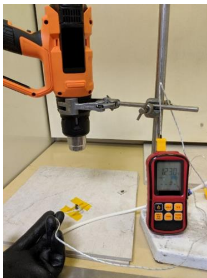
Figure S14: Photo of heat gun setup used for HAF annealing. Temperature was stabilised to 120 \pm 10 °C, confirmed with a thermocouple connected to a suspended substrate, matching the conditions during HAF annealing.
