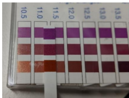
Figure S18: pH strip confirming pH of the undiluted np-SnO 2 to be ~11.5, with strong basicity due to KOH stabiliser.
