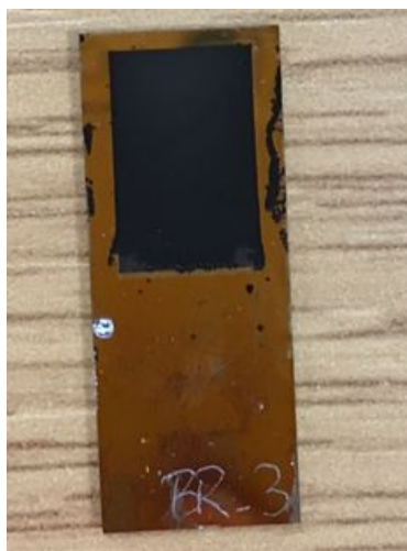
Figure S2. Image of the film electrodeposited by pulsed electrodeposition ( t_{\text{on}}=5\text{s} , t_{\text{off}}=10\text{ s} ) at -1 V vs. Ag/AgCl, with -1.3 C of the passed charge.
