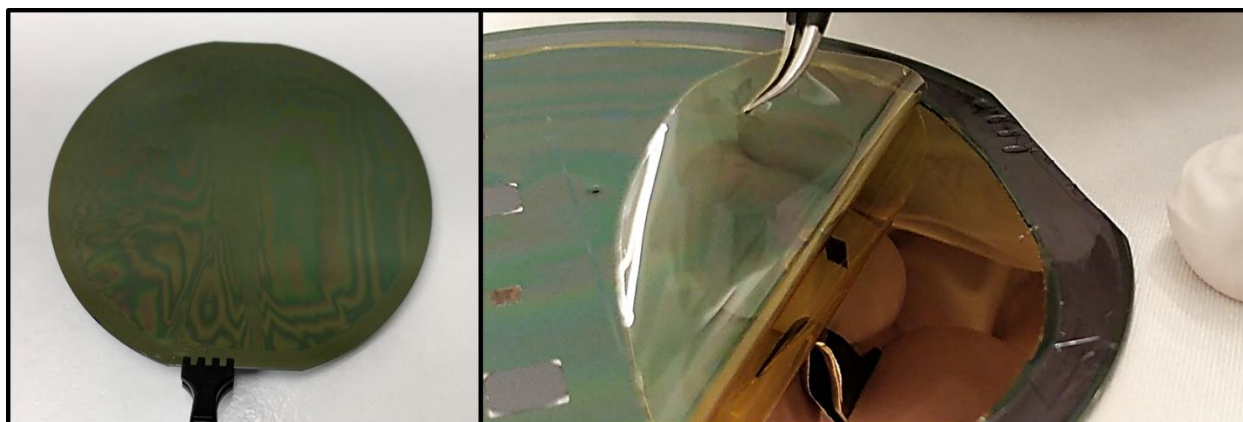
Figure S2. Polyimide thin layer coated on a 4-in silicon wafer and cured (left). Polyimide-based nanoporous membrane during the release from the wafer (right).
