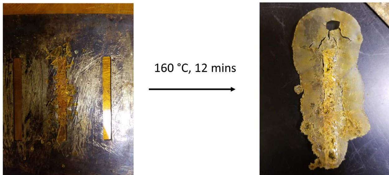
Figure S33. Attempted reprocessing of as-synthesized PU film without any catalyst present.
