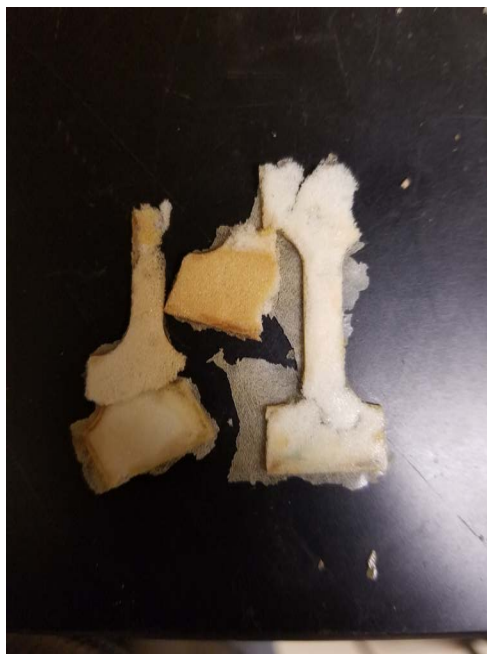
Figure S28. Attempted compression molding of catalyst-containing commercial PU foam showing poor processability.
