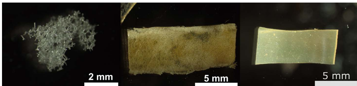
Figure S14. Optical microscopic images of commercial PU flexible foam (left), compression molded commercial PU foam (middle), and microcompounded commercial PU foam (right)
