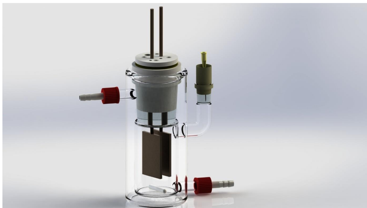
Scheme S2: Schematic picture of the beaker-type cell used in the scale-up reaction
