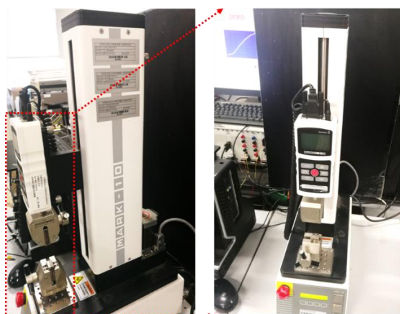
Fig. S14. Photographs of the uniaxial tensile tester for nanofiber films. Photo Credit: Xiao Peng, Beijing Institute of Nanoenergy and Nanosystems.
