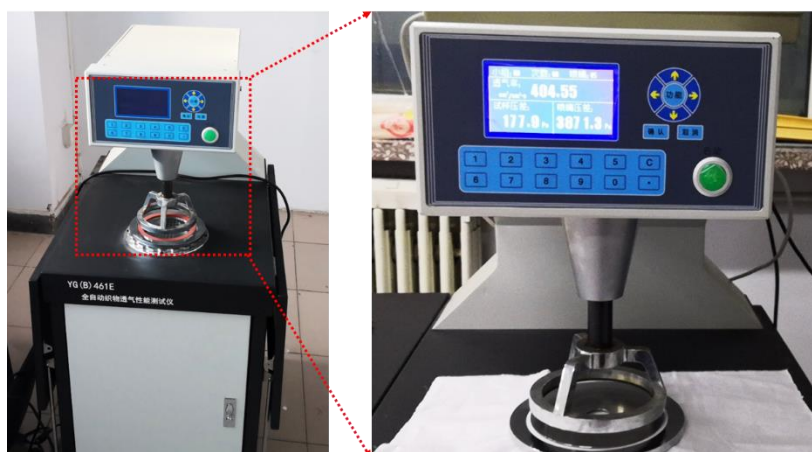
Fig. S18. Photographs of the air permeability tester for nanofiber films. Photo Credit: Xiao Peng, Beijing Institute of Nanoenergy and Nanosystems.
