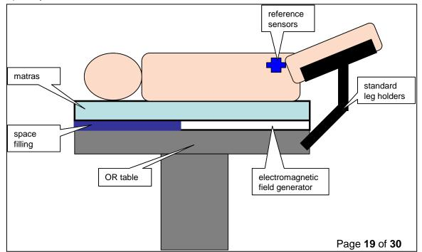
Figure 1: Schematic side-view of a typical patient setup for pelvic cancer surgery, combined with the Aurora navigation system
