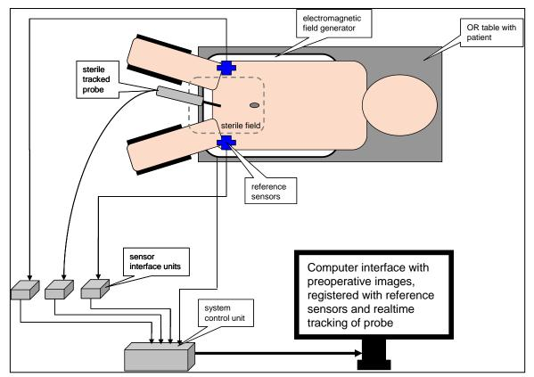
Figure 2: Overview of the navigation hardware components and the interconnections between the components
