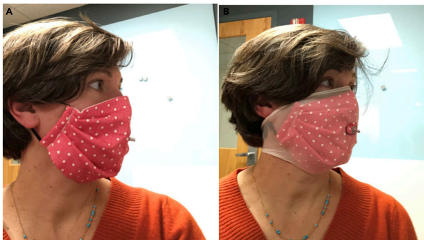
Figure 2. Example of Facemask and Nylon Overlayer Used in Tests
