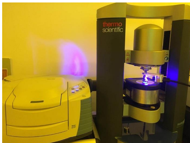
Supplementary Figure 3. Setup of ATR-FTIR and rheometer (blue light in the model was replaced by NIR light source in this case)
