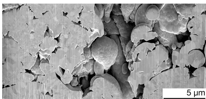
Figure S14: Laser-induced forward transfer of Cu and Au (LIFT).
