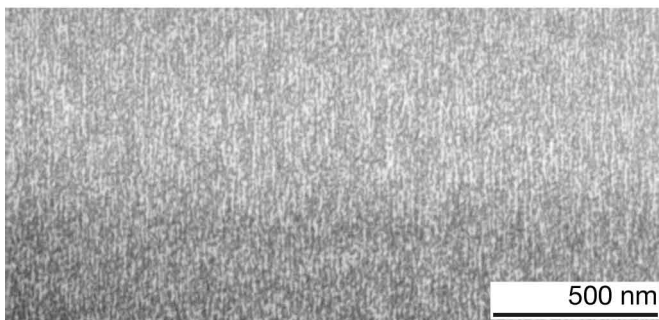
Figure S19: Focused ion beam-induced deposition (FIBID) of Pt (MeCpPt(Me) 3 ).
