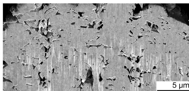
Figure S14: Laser-induced forward transfer of Cu and Au (LIFT).
