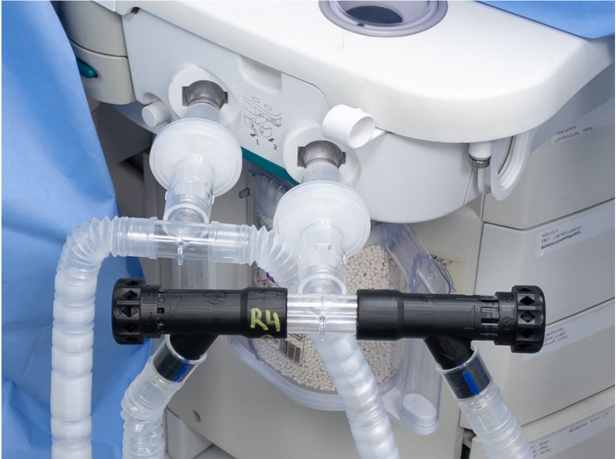
Figure 8 - Final assembled dual patient limbs connected to a GE Aisys Anesthesia Machine (also was tested with a Puritan Bennett 840 ventilator).
