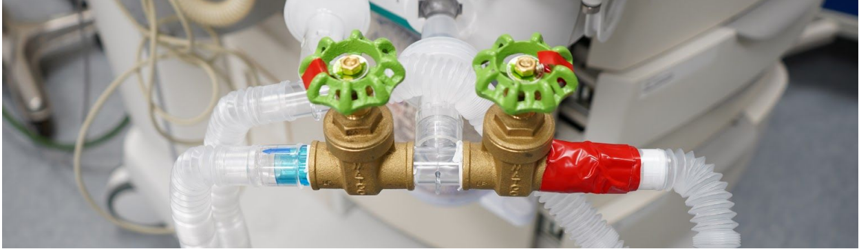
Figure 7 - Assembled Inspiratory Gate Check Valves. Note: red electrical tape (on right side) used to provide structural support, and colored labeling tape has been added to the valve on the right to indicate orientation.
