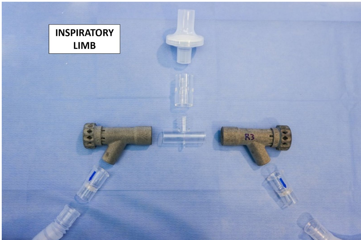
Figure 4 - Components of the inspiratory limb . The filter (top center) attaches to the ventilator inspiratory connection, while the one way valves (with blue arrows) connect to the inspiratory limb of the breathing circuit.
