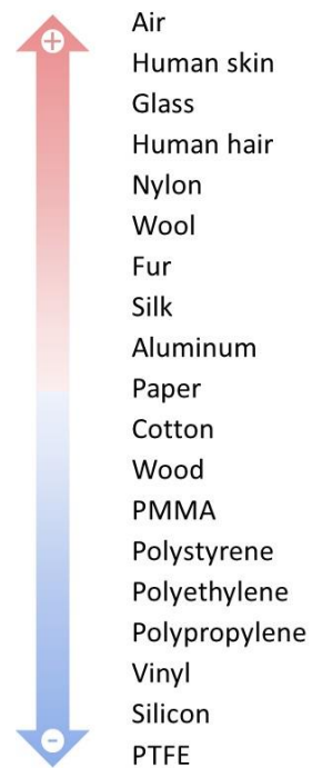
Supplementary Figure 1. Triboelectric series of various materials. “+” / “-” indicate whether a material tends to be positively or negatively charged when triboelectrification occurs. 1,2
