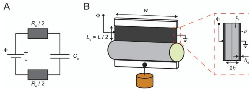
**Fig. S1.** Estimation of the RC time constant of Peano-HASEL actuators. (A) Equivalent circuit of a Peano-HASEL actuator. The actuator is modeled as two resistors  $R_e/2$  representing the resistance of the electrodes and a capacitor  $C_a$  representing the capacitance of the zipped region of the electrodes. (B) Definition of the parameters used to estimate the RC time of Peano-HASEL actuators.
