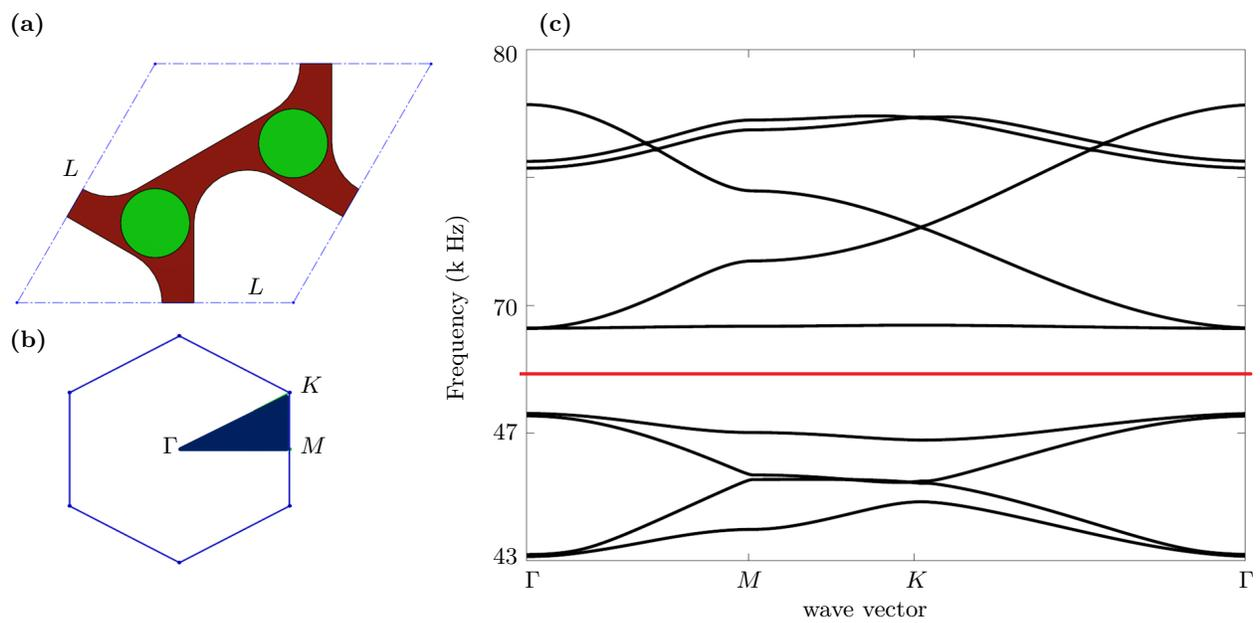
**Fig. S1.** (a) Schematic of the proposed hexagonal unit cell in this work (with the size of  $L$ ), composed of a PLA host layer with two bonded piezoelectric disks, (b) Schematic of the Brillouin zone of the proposed hexagonal unit cell, (c) Band structure of the hexagonal unit cell.
