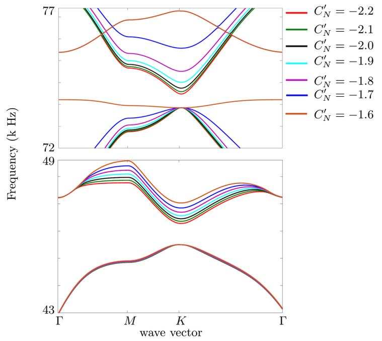
**Fig. S2.** (a) Schematic of a shunted piezoelectric disk and its connected circuit. (b) Band structure of the hexagonal unit cell for different values of negative capacitance plotted for two different ranges of frequency.
