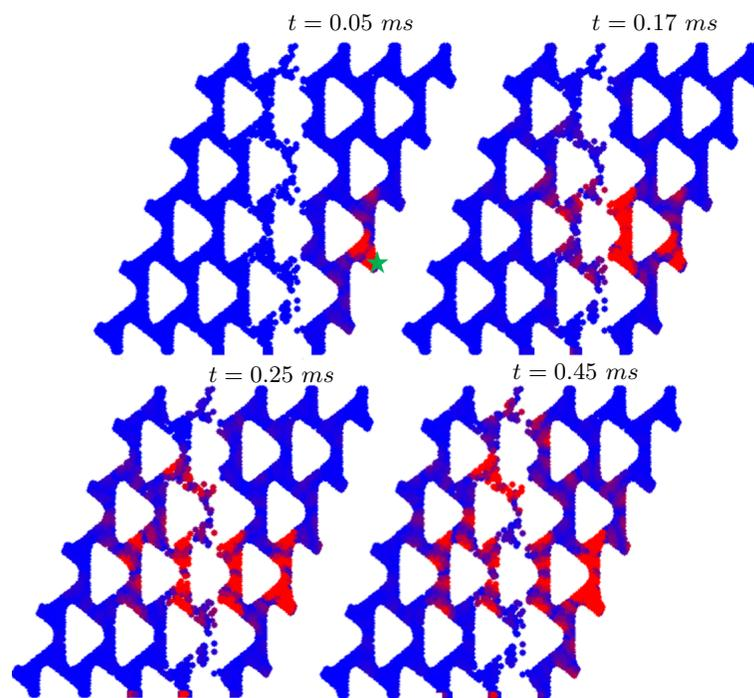
**Fig. S7.** Experimentally measured displacement field of the system with a sharp-angled interface (depicted in Fig. 4(b) of the manuscript) captured at different times, excited by a source with frequency  $77 \text{ kHz}$ . The source location is marked with a green star.
