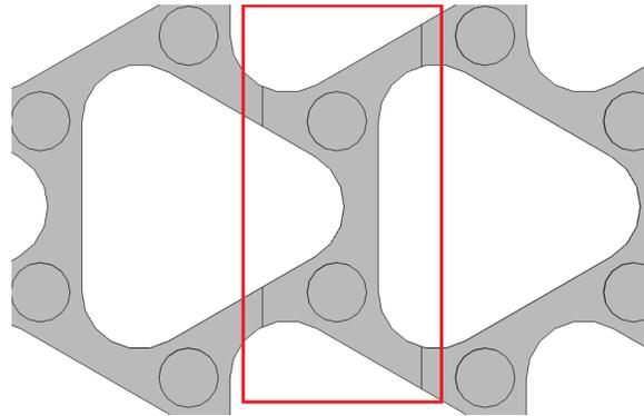
**Fig. S4.** A schematic of the considered control volume to calculate the amount of standing waves.
