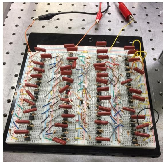
**Fig. S5.** Fabricated experimental setup. On the left: the tested structure wired to the external circuits. On the right: the external circuits used to provide negative capacitance.
