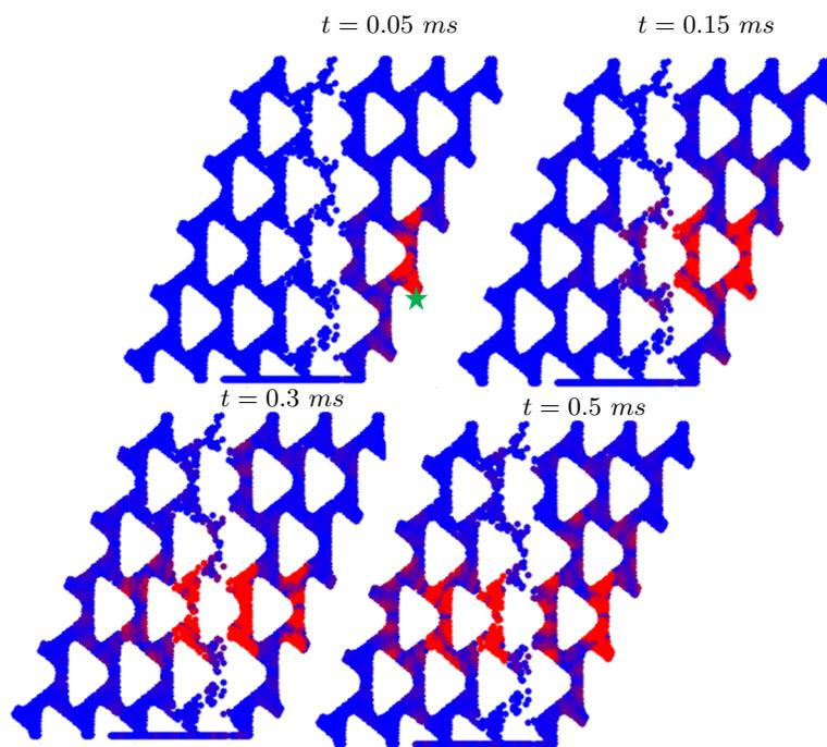
**Fig. S6.** Experimentally measured displacement field of the system with a horizontal interface (depicted in Fig. 4(b) of the manuscript) captured at different times, excited by a source with frequency  $77 \text{ kHz}$ . The source location is marked with a green star.
