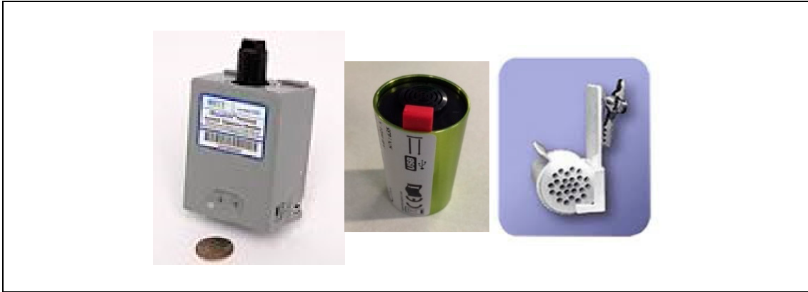
Figure S1. Wearable sensors used in the study: RTI MicroPEM (left), Cairpol CairClip (middle), and Ogawa O 3 passive sampler (right)
