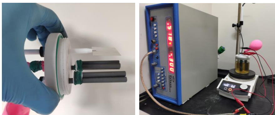
Supplementary Figure 3. 10 mmol scale Electrolysis setup
