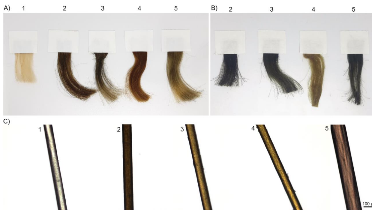
Figure S1. Blond, human hair purchased from a second vendor (Emosa) was dyed using polydopamine formulations (companion to Figure 1 , main text). A) Photographs of hair before (1) and after dyeing at room temperature for 2 h using 3% \text{NH}_4\text{OH} (2), 0.05 N \text{NaOH} (3), 10 mM \text{CuSO}_4/1 M \text{H}_2\text{O}_2 (4) and Tris buffer pH 8.5 (5). B), as for A), but the dyeing was conducted at 37-40 °C. C) Optical micrographs of individual hair fibers dyed at 37-40 °C (panel B).
