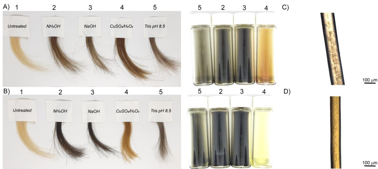
Figure S5. Photographs of hair before (1) and after dyeing with polydopamine using 3% \text{NH}_4\text{OH} (2), 0.05 N \text{NaOH} (3), 10 mM \text{CuSO}_4/1 \text{ M H}_2\text{O}_2 (4) and Tris buffer pH 8.5 (5). Dyeing was carried out for 2 h at A) room temperature and B) 37-40 °C. The colors of the resulting polydopamine solutions in which the hair was suspended, are shown in vials. C) Optical microscopy images of an untreated blond hair fiber (sample 1 in panels A-B) and D) hair dyed using 10 mM \text{CuSO}_4/1 \text{ M H}_2\text{O}_2 at 37-40 °C (Sample 4 in panel B).
