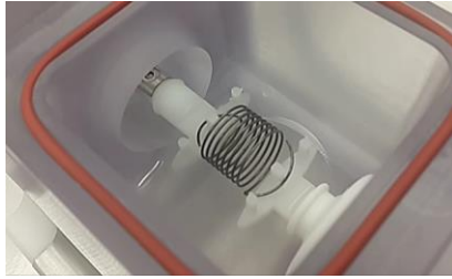
Supplementary Figure 8. Picture of the instrumentation spring housed with the bioreactor culture chamber for the load cell characterization tests.
